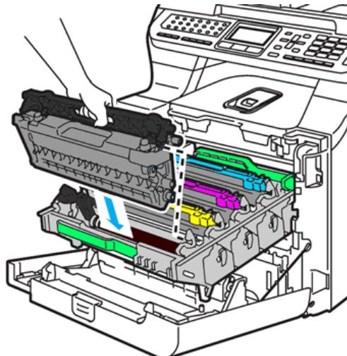
If the toner runs out or the toner cartridge/ drum unit comes to the end of its life, separate the toner cartridge and drum unit and replace the unusable consumable only.
