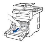
4. Hold the handle of the toner cartridge and gently push it away from you to unlock it. Pull it up and out of the drum unit. Repeat this for all toner cartridges.
