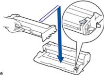
6. Put the toner cartridge firmly into the new drum unit until you hear it lock into place
