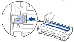
Be sure to return the tab to the Home position (**1**). The arrow on the tab must be aligned with the arrow on the drum unit. If it is not, printed pages may have a vertical stripe.
