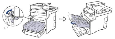
Hold the green handles of the drum unit when you carry it. DO NOT hold the sides of the drum unit.
