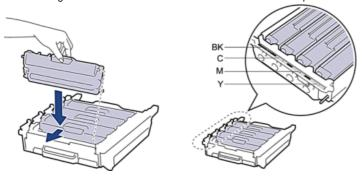
Make sure you put the toner cartridge in correctly or it may separate from the drum unit.
