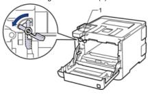
10. Gently slide the drum unit into the machine until it stops at the green lock lever.
