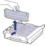
8. Reinsert the toner cartridge into the new drum unit and gently pull it toward you until you hear it lock into place. Make sure that you match the toner cartridge colour to the same colour label on the drum unit. Repeat this for all toner cartridges.
